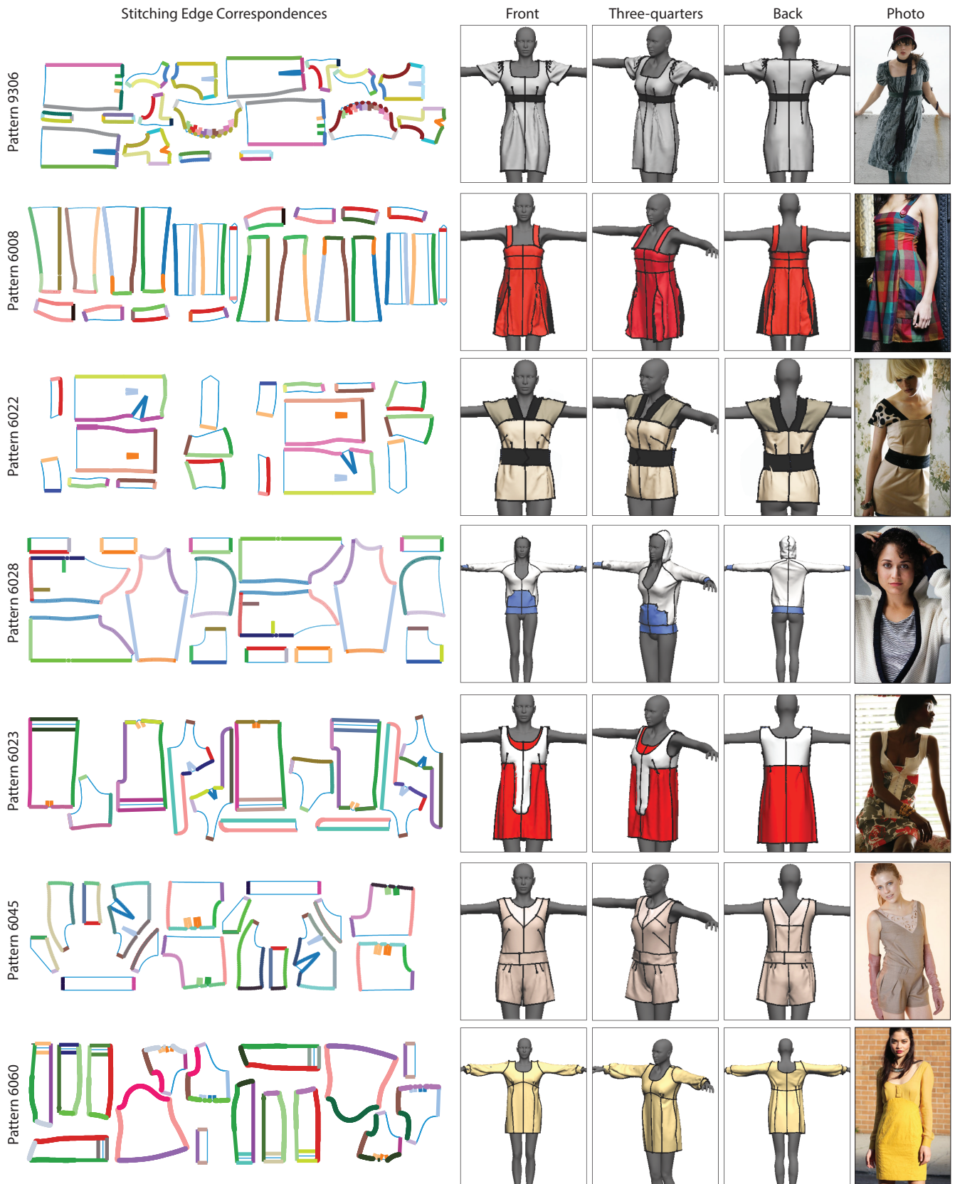
Figure 6: Parsing and simulation results for 7 sewing patterns. For each pattern we color-code the stitching edge correspondences identified by our parser. We show three views of the 3D garment model draped on a mannequin using our simulator. For comparison we include a photograph of the garment from burdastyle.de . Note that our parser correctly identified all of the stitching edge correspondences for the garments shown in this Figure.
